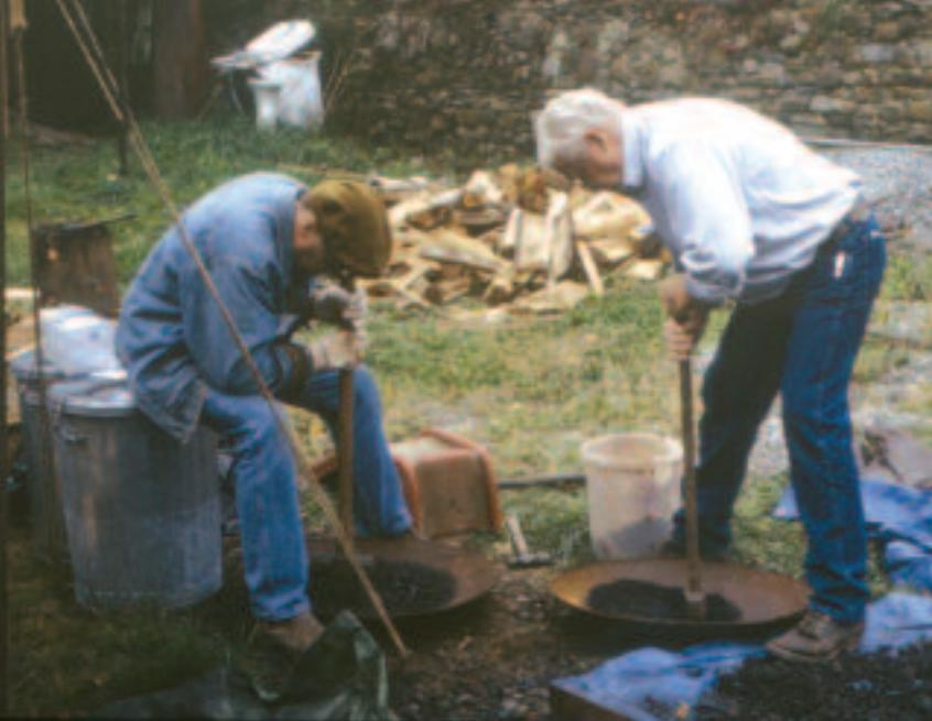
Before smelting can begin, the ore needs to be broken up into fragments about the size of half a pea.
