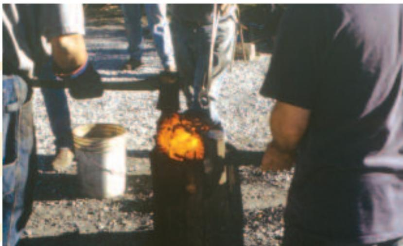
We carry the bloom to a hollowed log and split the bloom using an axe pounded by sledgehammers. To preserve its temper, the axe must be quenched frequently while it splits the still-hot bloom.
