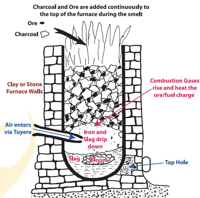
This generalized low-shaft furnace shows how hot gases rise and pre-heat the ore/charcoal charge. Oxidation takes place where the hot air and charge meet. During the smelt, the slag can be tapped to drain out, but to remove the bloom the furnace wall must be broken (adapted from p. 29 of William Rostoker and Bennet Bronson. *Pre-industrial Iron: Its Technology and Ethnology*. Philadelphia, PA: Archaeomaterials, 1990).
