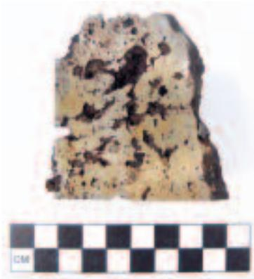
Sliced open, the iron in our bloom is easy to see, as are the air holes that a blacksmith will have to hammer closed.
