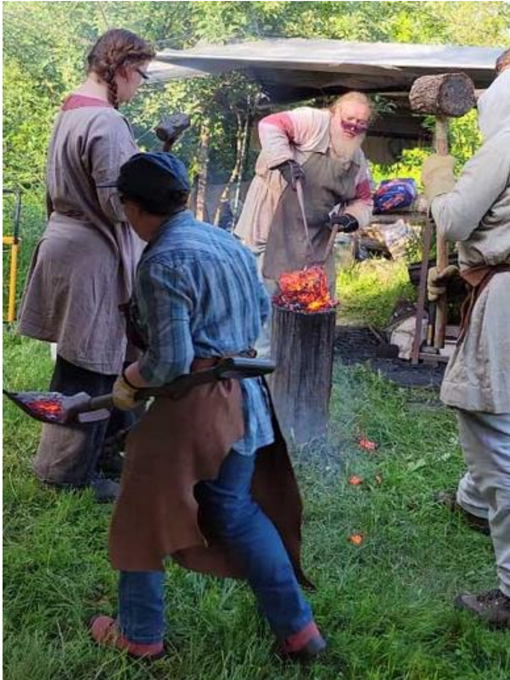
(figure vii) At the end of the second round of hammering, the mass being shifted to expose a different side for hammering. Roughly fist sized pieces of slag bowl are being moved clear of the work area, while several (hot!) egg sized fragments can be seen still on the ground to the right.
