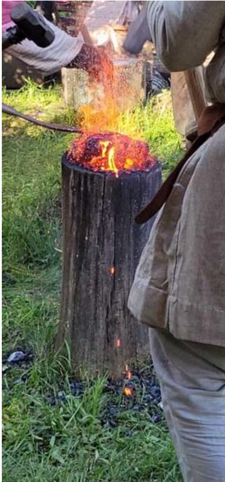
(figure viii) About half way through the compaction process, the bottom of the bloom now uppermost. Hammering has cracked open an internal pocket, ejecting liquid slag, which can be seen running out and dribbling as small pieces down on to the ground.
