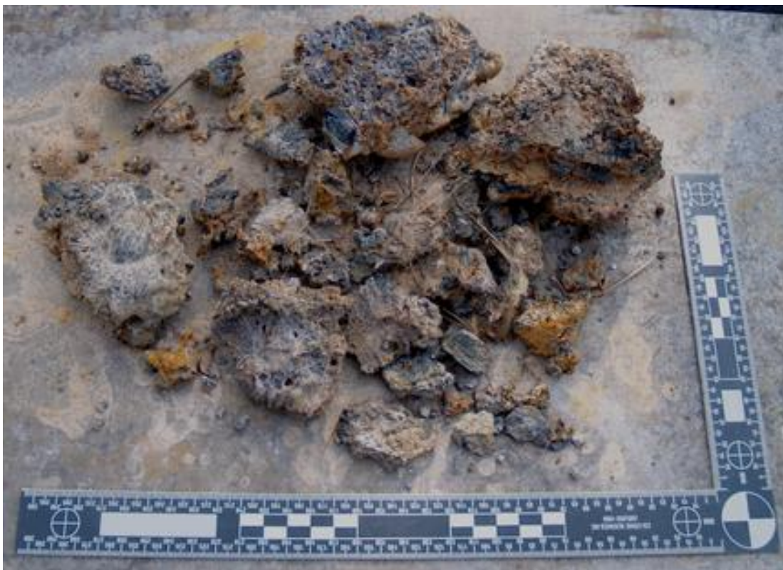
(figure iii) Slag Bowl fragments - the pieces above were gathered while hot and dropped into a water filled bucket (for safety), resulting in some pieces shattering and some fast surface rusting.
