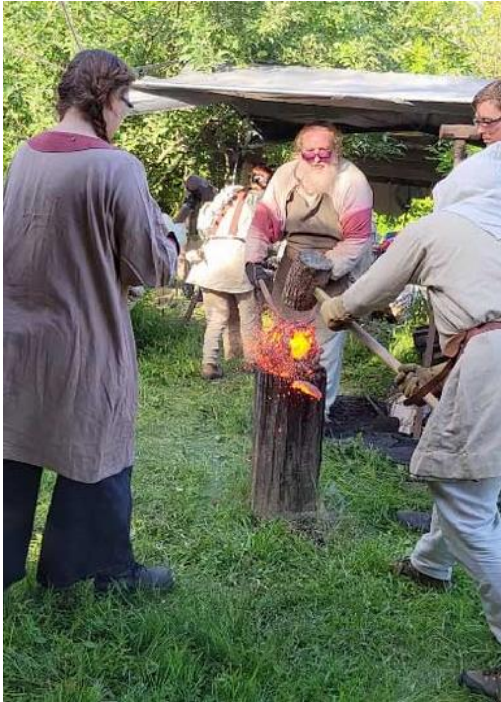
(figure vi) Part way through the first hammering sequence. In this case the entire slag bowl encasing the bloom was extracted, resulting in a much larger starting block than is typical for this team, about 25 cm in diameter and 20 cm top to bottom. A large piece of encasing slag bowl material can be seen flaking off, exposing the much hotter metallic bloom surface underneath.
