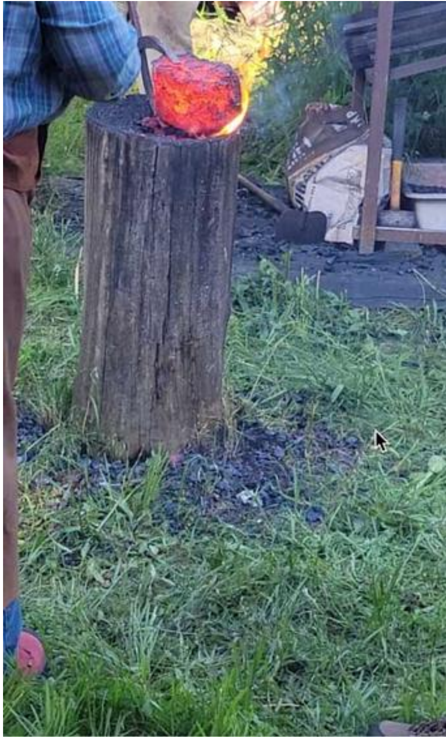
(figure x) At the end of the initial compaction sequence. The bloom at this point has been formed into a rough cube through repeated hammering, but has cooled down below a temperature where any further work would be effective without re-heating (actually into a 'red' colour to the eye). Even with repeated removal of the larger hot pieces of slag that had been broken away, the circle of debris created is obvious.
