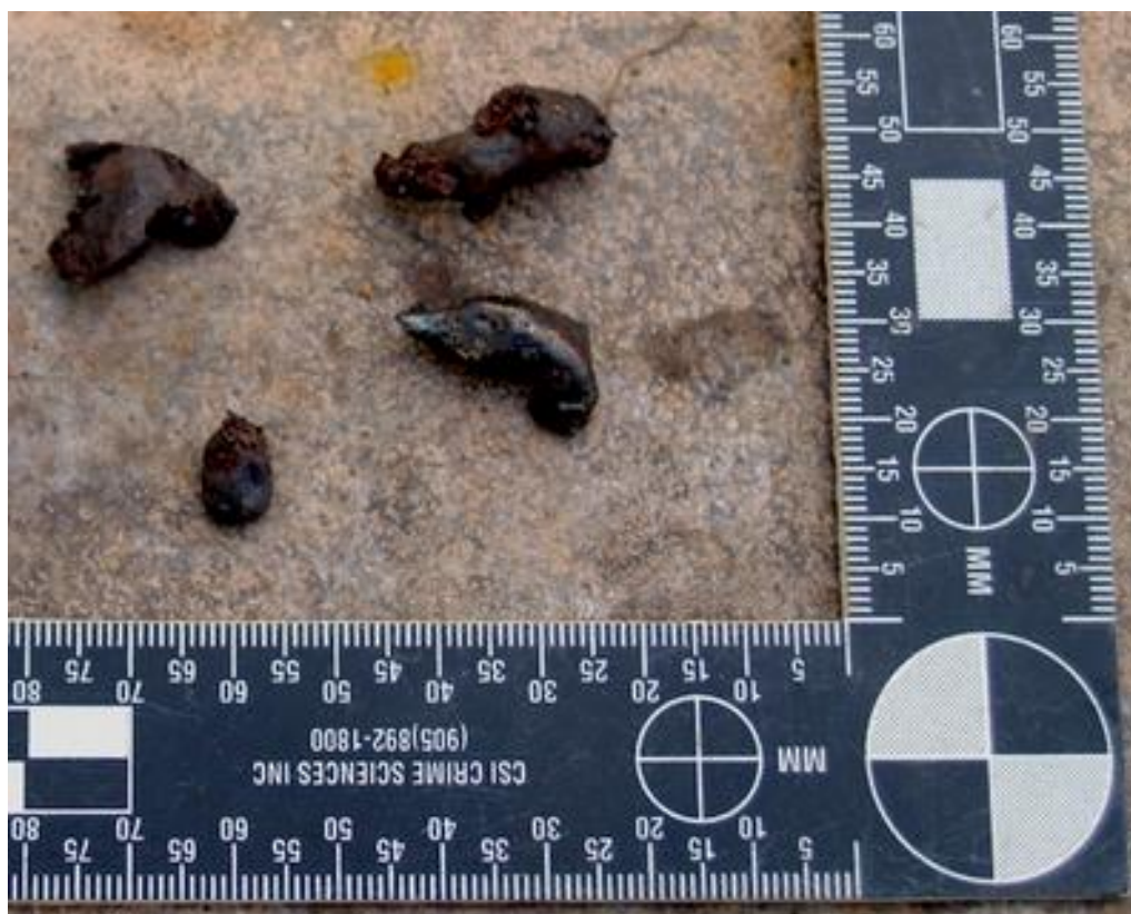
(figure v) Liquid Slag droplets – collected from the base of the stub, with dark coloured and smooth ‘melted’ looking surfaces.
